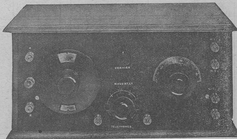
A view of the finished receiver. The large dial is that of the variometer.
